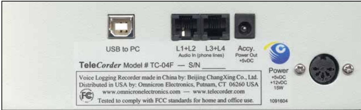
**TeleCorder rear view, showing USB jack for connecting to a computer, two modular phone jacks for connecting to the source of the conversations to be recorded, 5vDC jack to power accessories, and DIN connector for connecting to output of the supplied AC power adapter.**
